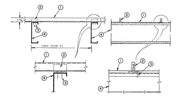
1. Metal Roof Deck Panels \* — No. 22 MSG or No. 24 MSG min thickness coated steel panels. Panels 12 in. wide, 1-3/4 in. high at the ribs. Panels continuous over two or more spans. A bead of sealant may be used at panel side joints.
